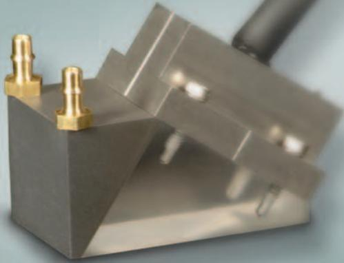
At Blatek, we have developed a line of custom phased array transducers that are based on our piezo-composite and proprietary double matching layer design that produces 80% plus bandwidth and maximized sensitivities. We offer linear, curved linear, annular, 1.5D and 2D matrix array capabilities.
